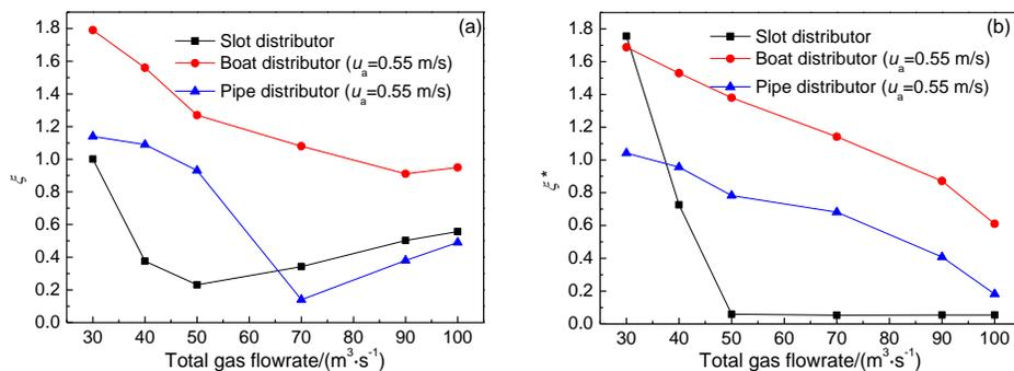
Fig. 2 Comparison of heterogeneity indices of the three spent catalyst distributors
