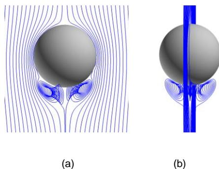
Figure 1. Streamlines around the particle with gas velocity of 0.5m/s and liquid velocity of 0.24m/s at
