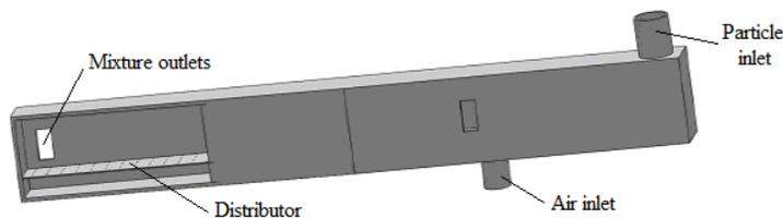
Fig. 1 Schematic of the mechanism of the tested model of the new slot catalyst distributor
