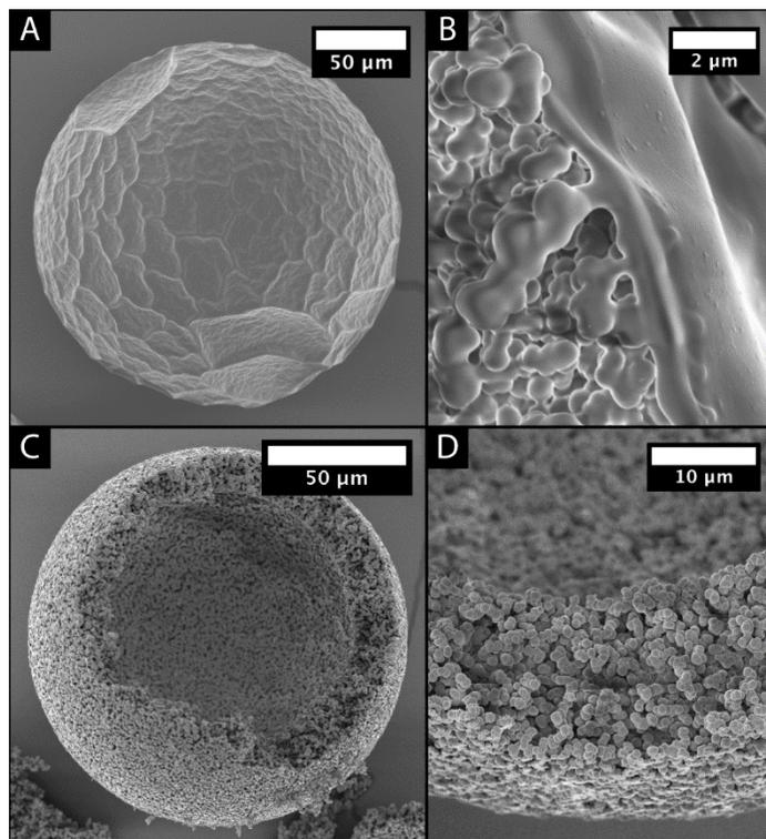
Figure 2 – A and B: Skin formation on capsules produced with 35 wt % of diisodecylphthalate. C and D: Open porous structure on capsules produced with 30 wt % undecanol.
