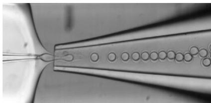
Figure 1. Synthesis of poly(tert-butyl acrylate) microcapsules using a combination of alumina nanoparticles and surfactant as stabilizers.
