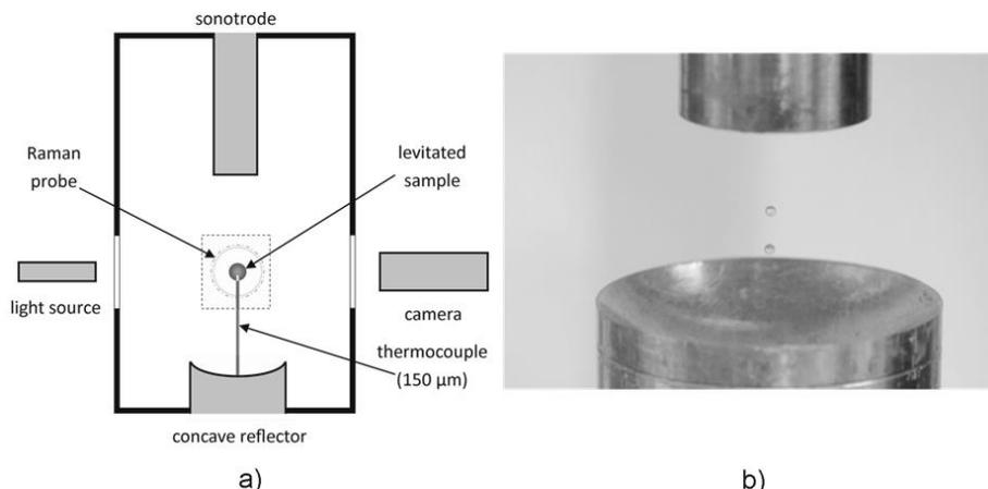
Figure 1 – a) Process chamber of the acoustic levitator with the Raman probe in the background outside the chamber, b) levitated mannitol-water droplets.
