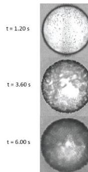
Figure 3. Oil droplets in water, stabilized by alumina nanoparticles at increasing residence time in a microfluidic channel.
