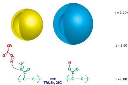
Figure 2. Hydrolysis of poly(tert-butyl acrylate) microcapsule to form poly(acrylic acid) hydrogel microcapsule.
