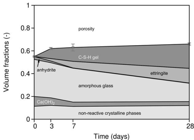
Figure 1 – Volumetric model of phase evolution during hydration of activated CFBC fly ash
