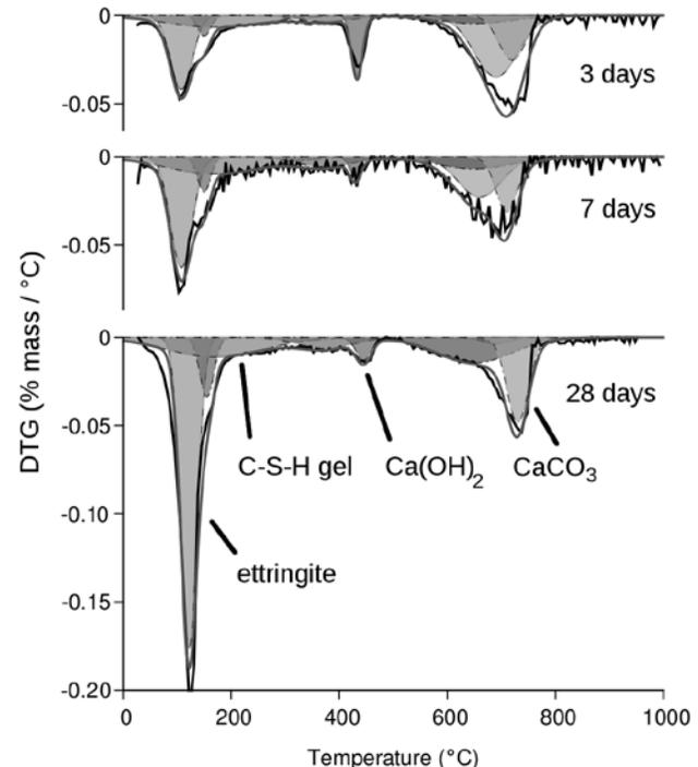
Figure 2 – Deconvolution of DTG curves of CFBC fly ash pastes for different ages and identification of phases
