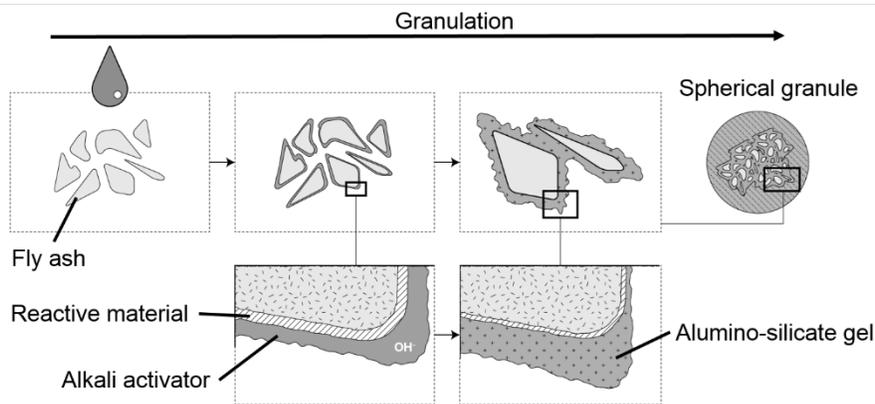
Figure 1 – Descriptive diagram of the granulation-alkali activation process
