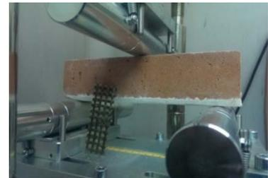
Three point Flexural Test of EB FRGP reinforced Brick (Basalt fabric)
