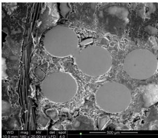
SEM image of steel fibers fabric embedded in geopolymer matrix
