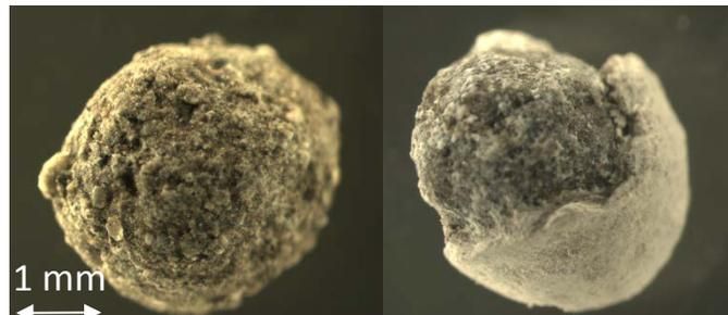
Figure 2 – Microscope images of geopolymer granules. On the left image is an alkali activated fly ash lightweight aggregate. On the right image is a fly ash geopolymer granule coated with alkali activated metakaolin.
